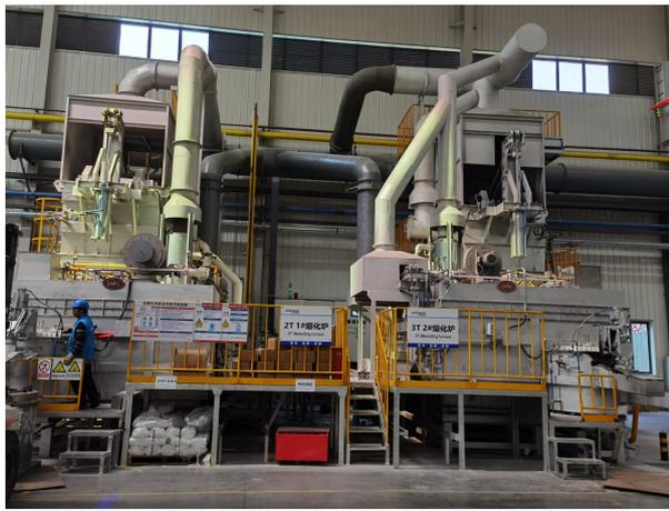
熔化废气集气罩
